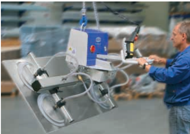
Handling of aluminium sheets with a VacuMaster Basic, 250 kg, 90° swivelling
