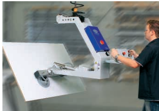
Handling of coated sheets of wood with a VacuMaster Comfort, 75 kg, 180° turning
