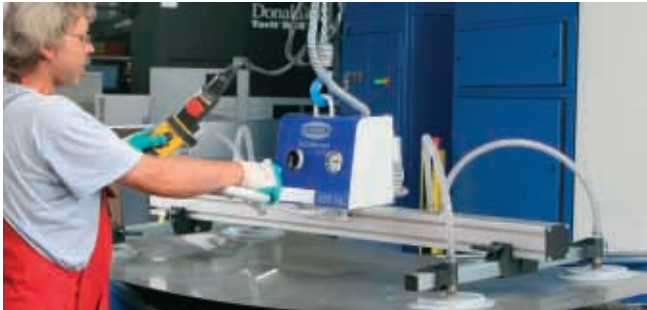
VacuMaster Basic, maximum load 250 kg, horizontal
