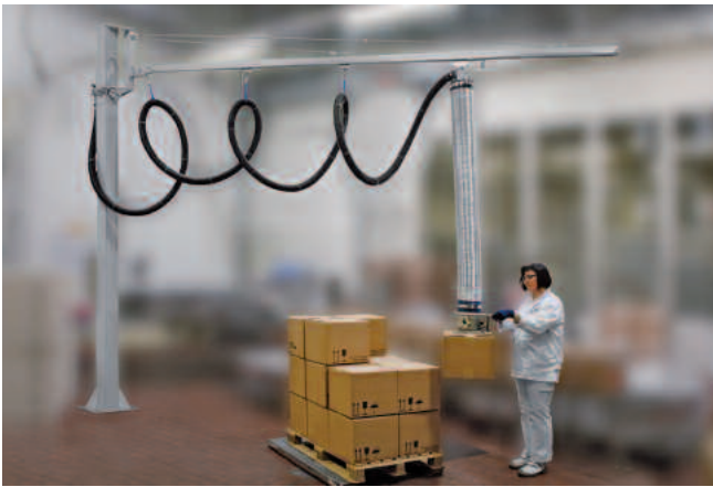
Column-mounted slewing crane with steel crane rail for zones with a risk of explosion, 110 kg load, 4 m jib length
