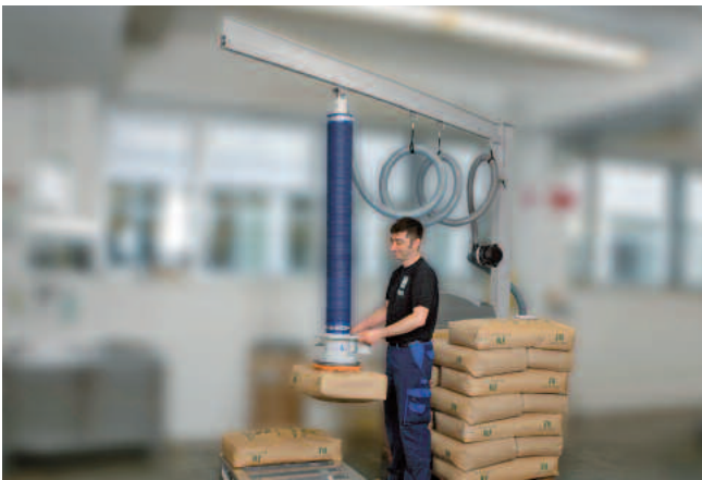
Column-mounted slewing crane with steel rail and flat jib, 85 kg load, 3.5 m jib length
